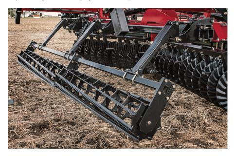
The patented TigerPaw™ Crumbler has two edges to attack large clods twice and tuck residue in the surface. It provides more uniform clod sizing and residue distribution, providing for a level finish and better seed-to-soil contact in the spring. Available with either the simple to use value spring down pressure option or hydraulic down pressure.
