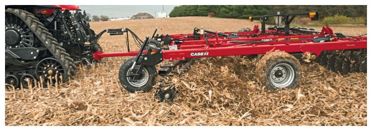
The geometry of the 18° gang angle coupled with the shallow concavity blade ensures that the blade's angle of attack is always vertical so that the blade always runs on it's edge. This combination causes soil to explode off of the front side of the blade while maintaining minimal back-side blade pressure, resulting in maximum soil penetration in tough conditions and reduced sub-surface compaction when compared to competitive vertical tillage tools.
